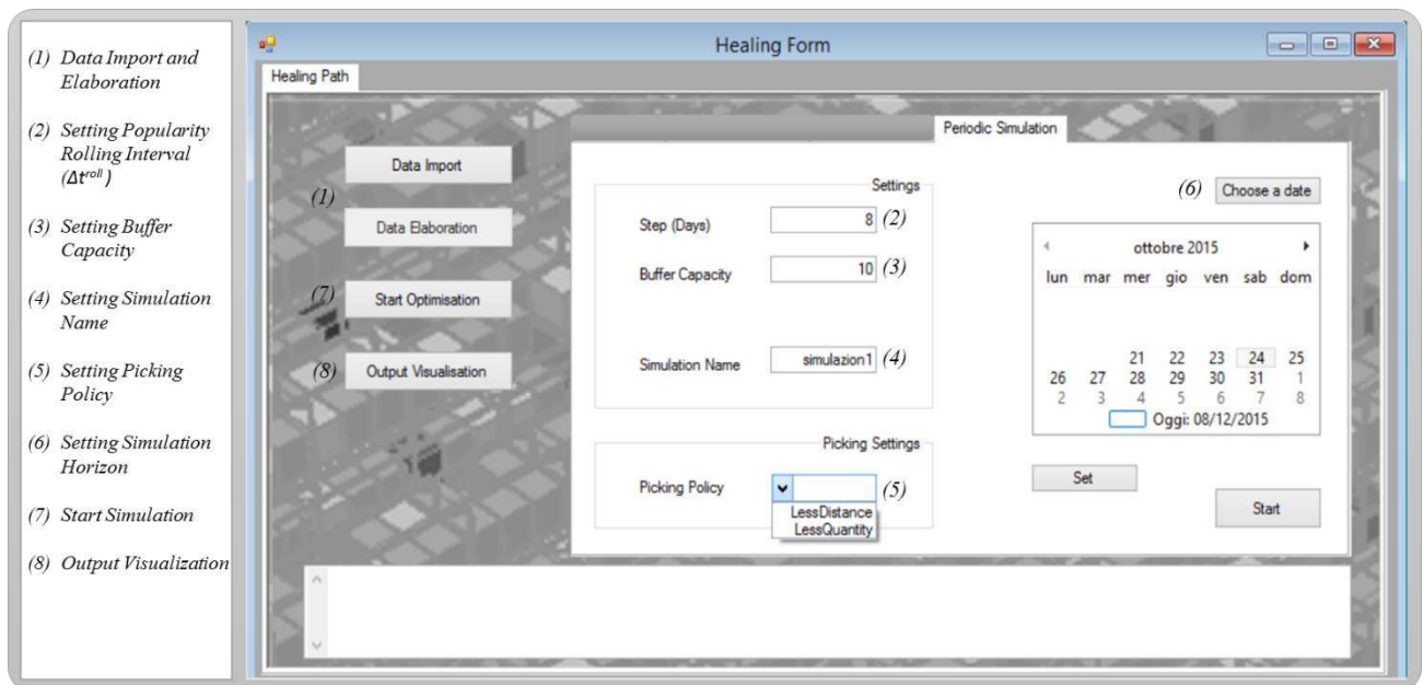
Figure 2. Graphic user interface of the simulation tool implementing the adaptive policy
