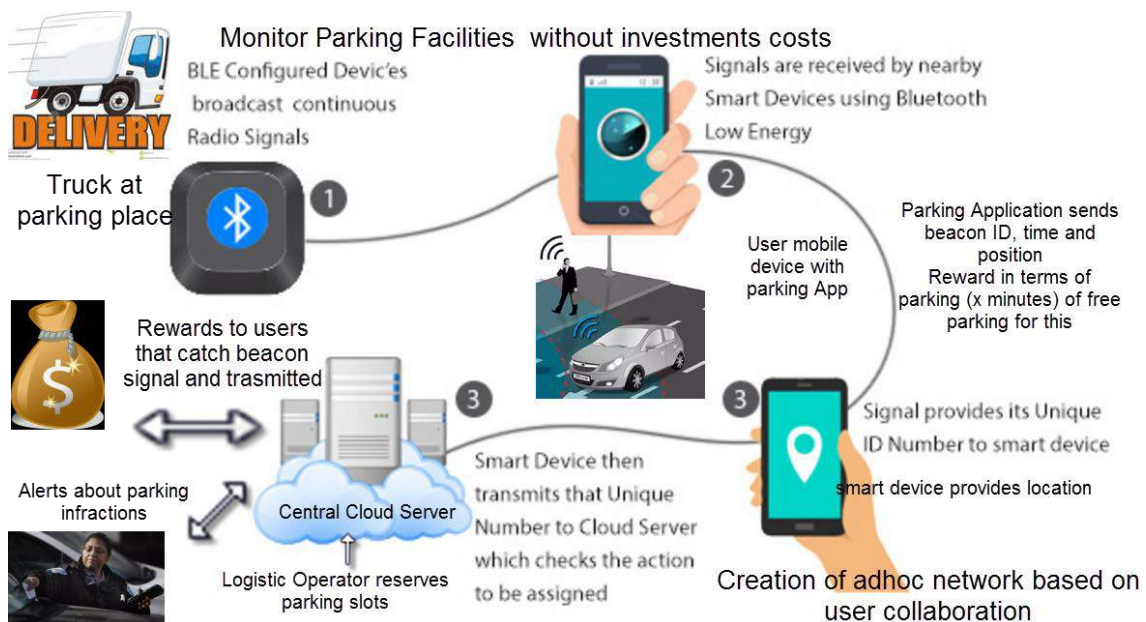
Figure 2. Overview of the proposed approach to create parking monitor facilities without investments costs using an ad-hoc network of user mobile devices in a collaborative process
