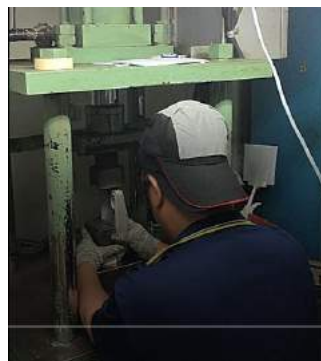
Fig. 2 The operation of hydraulic shaping machine.
